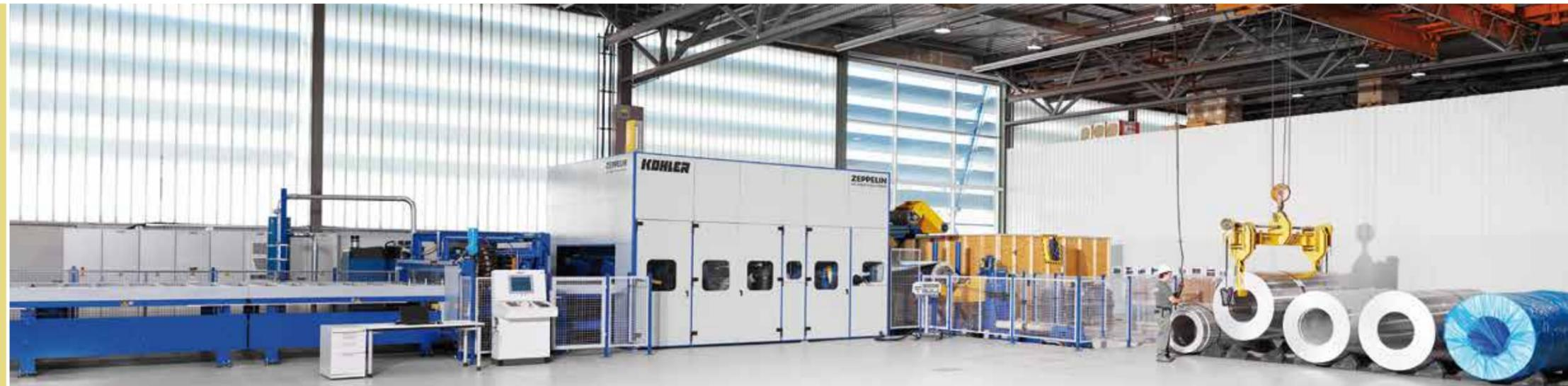
High degree of automation: Special production plants for silos in compact design ensure maximum, consistent quality and short delivery times.
