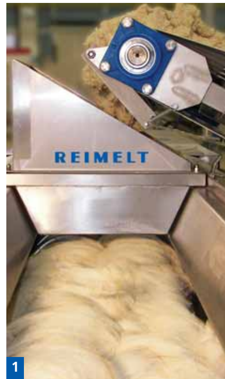
Picture 1: Product transfer from the Codos®Mixer to the Codos®Kneader
