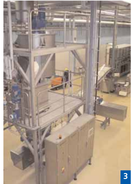
Picture 3: Codos®System with dry materials mixer
