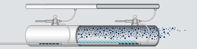
**Airfloat:** stainless steel pipes; air injection through slots to avoid dead spots in the conveying of critical products such as silica.
