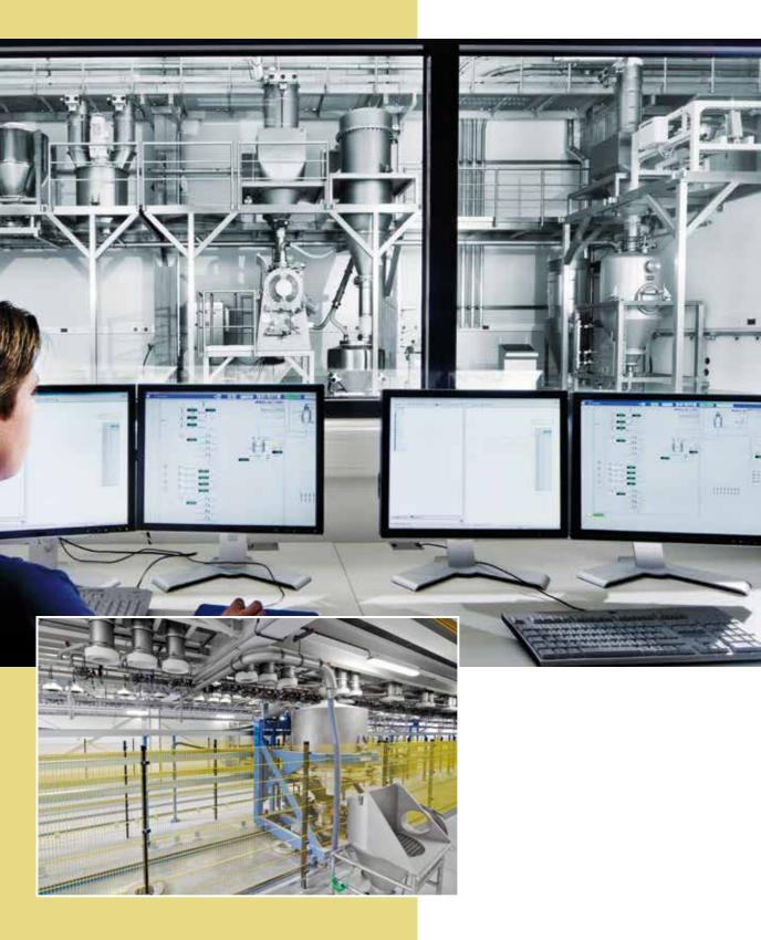
Manual weighing is a thing of the past: at Zeppelin, minor chemical components are automatically weighed. The individual components are dosed directly into the bag without needing any other intermediate vessel. This means: highest precision in the recipe, no impurities and no human error. Naturally, the bags can be printed on directly for later processing.
