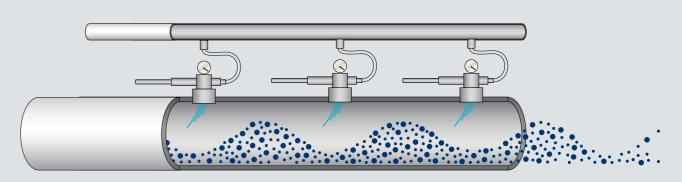
**Overflow:** PE or stainless steel pipes; air injected at points every 0.5 to 1.0 m distance. For sensitive powdery products such as carbon black, etc.
