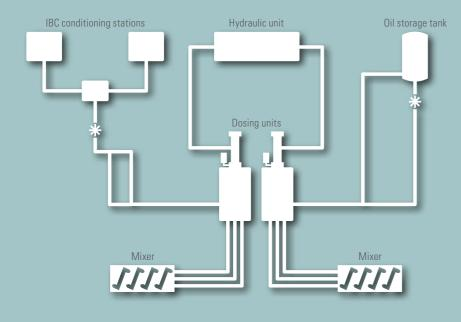
You hold all the aces with Zeppelin's newly developed liquid dosing system: quick assembly, versatile, customized to your requirements, safe operation and highest degree of cleanliness in daily use.
