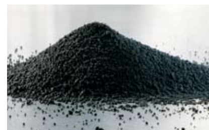
Carbon black with a minimum fines content after optimized conveying
