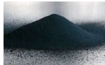
Carbon black with high fines content after conveying with too high a velocity
