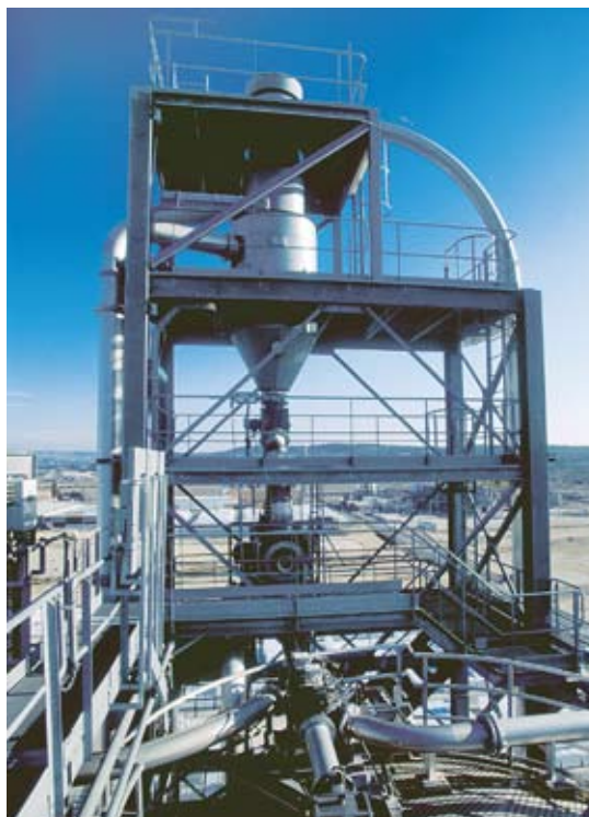
Innovative technology for purification of the product: from the drum sieve via the elutriator to the cyclone.
