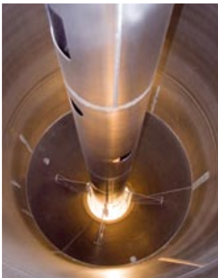
Left: Interior view of a Centro-Blend and its central blending pipe
